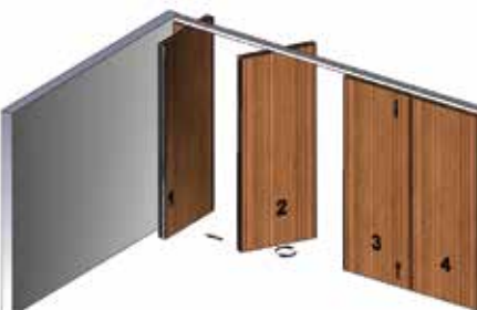
Pic. 9: Example of the panel movement with a single point suspension.
